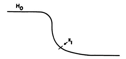
Fig. 1. Temperature distribution in cooling wave.
