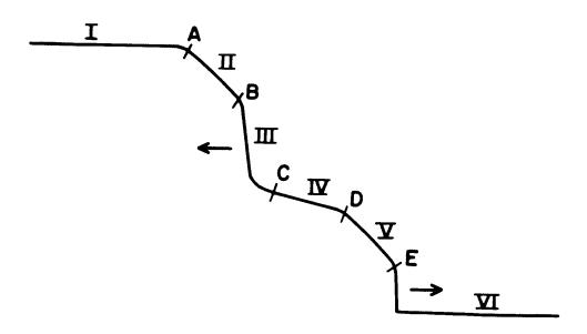
Fig. 2. Schematic temperature distribution. I, isothermal sphere; III, cooling wave; VI, undisturbed air; E, shock front. II, IV, and V are expanding adiabatically.
